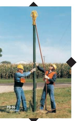
asily operated by one man, Rhino Post Drivers deliver up to 1700 blows per minute. One moving part, a reciprocating piston, strikes directly on the Post or Drive Cap. The Drivers have low air consumption rates, are light-weight and hand portable, ideal
